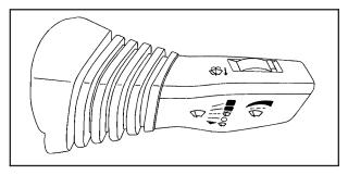
The lever on the right side of the steering column operates the windshield wipers. Push up or pull down on the lever to place it in one of the following positions.  $\mathbf{W}$  (Mist): Pull the lever down and release it for a single wiping cycle. The lever will return to its original position. For more cycles, hold the lever down before releasing it.
